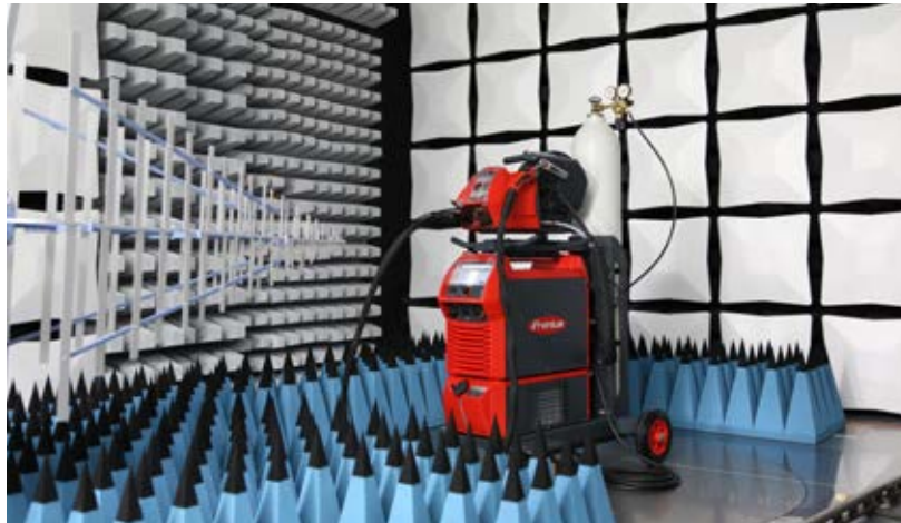
Picture 1: Test of the electromagnetic compatibility of a welding power source
