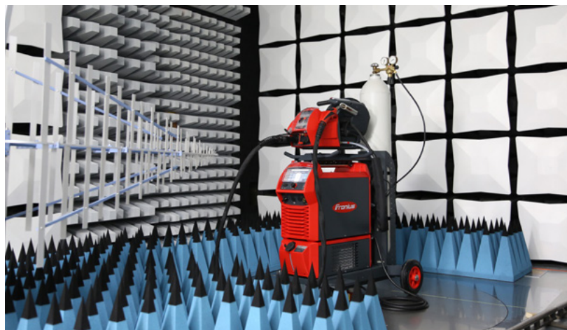
Figure 1: Testing the electromagnetic compatibility of a modern welding power source
